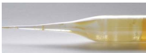
Fig. 4. Single crystals of \text{PbX}_2 grown by vertical Bridgman method, sealed in gaseous \text{X}_2 atmosphere: (a) \text{PbCl}_2 ; (b) \text{PbBr}_2 .
