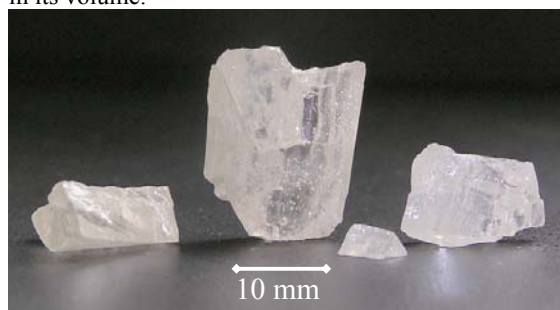
Fig. 3. \text{PbBr}_2 crystals obtained (from previously halogenated source material) by zone refining in gaseous \text{Br}_2 flow – after four passes.
